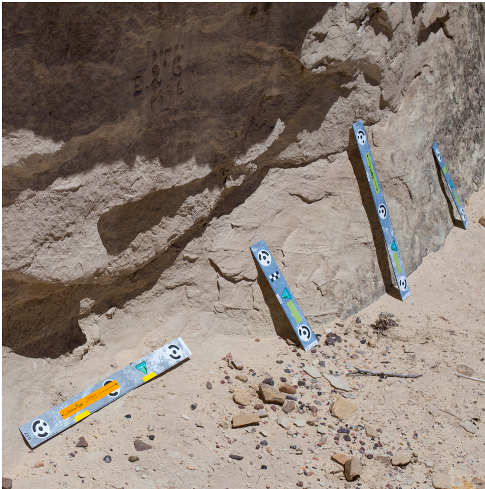
Figure 3: Four scale bars in place near an area of rock art and inscriptions to be imaged. These scale bars are placed near, but not covering, the inscriptions that appear above them on the rock.
